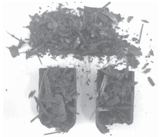
Figure 7. Cross-sectional views of crushed tubes under dynamic condition
